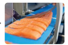
2. The fillet is cut into slices with highspeed precision and then realigned to enter the BC 100.
