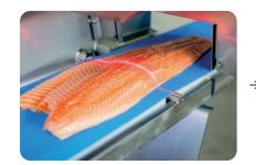
Salmon fillets enter the BC 225S and are scanned for the best cut configuration.
